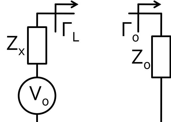
The source (eg. the transistor) having  $Z_x$  needs to see a certain reflection coefficient  $\Gamma_L$  towards the load  $Z_o$
