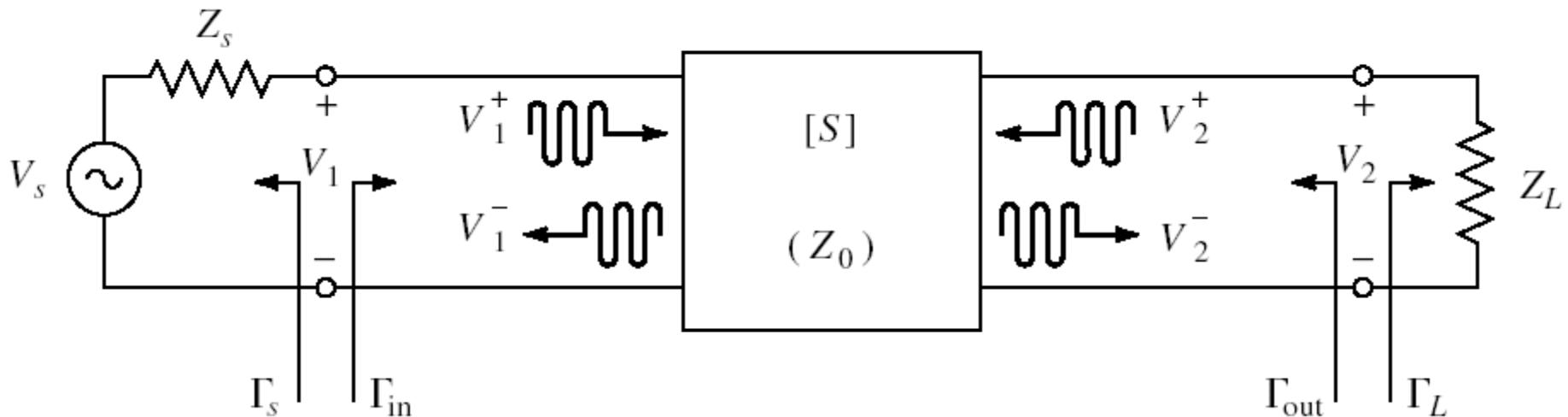
$$\Gamma_{in} = \frac{V_1^-}{V_1^+} = S_{11} + \frac{S_{12} \cdot S_{21} \cdot \Gamma_L}{1 - S_{22} \cdot \Gamma_L}$$
